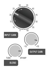
On vocals, try using the TUBE path for an intimate vocal, balance the INPUT GAIN and OUTPUT GAIN to accentuate a proximity effect on a condenser mic.
